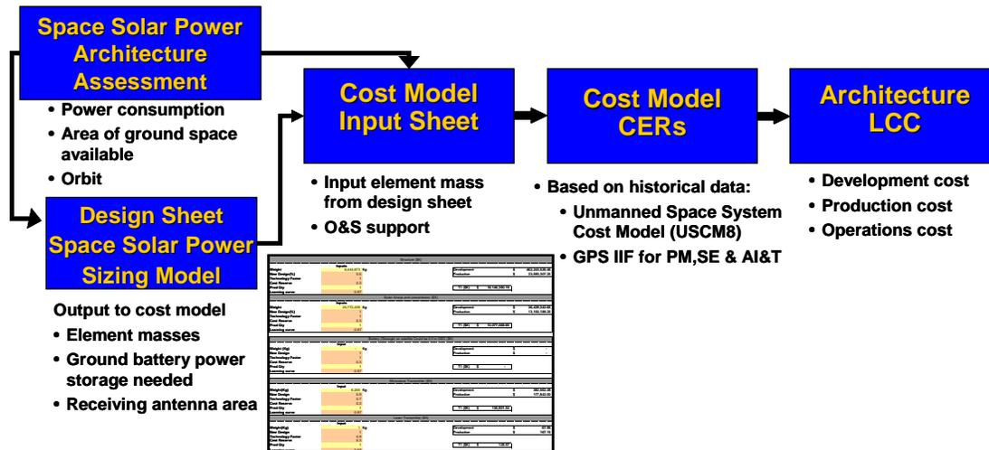
**Figure 6. Cost model process flow overview. Design Sheet mass outputs, architecture structure, and model inputs are used to determine element costs.**
