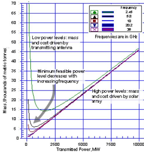
**Figure 7. Notional GEO SPS mass for several power beaming frequencies.**
