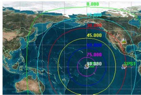
Figure 10. Elevation angle contours for a geostationary SPS at 150° west longitude. An SPS at this location can beam power to the west coast of the United States and Mexico, while maintaining a reasonable separation from presently operational geostationary communications satellites.
