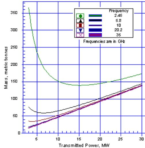
**Figure 8. Notional masses of small SPS's in a 350 km low Earth orbit. Such an SPS can supply power to forward military bases.**
