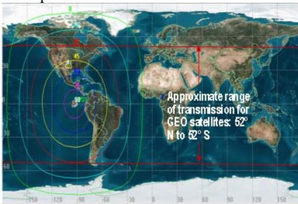
Figure 9. Elevation angle contours for a geostationary SPS at 90° west longitude. Even with a minimum elevation angle of 30°, most of the world's population can be served by solar power satellites in the geostationary orbital belt.
