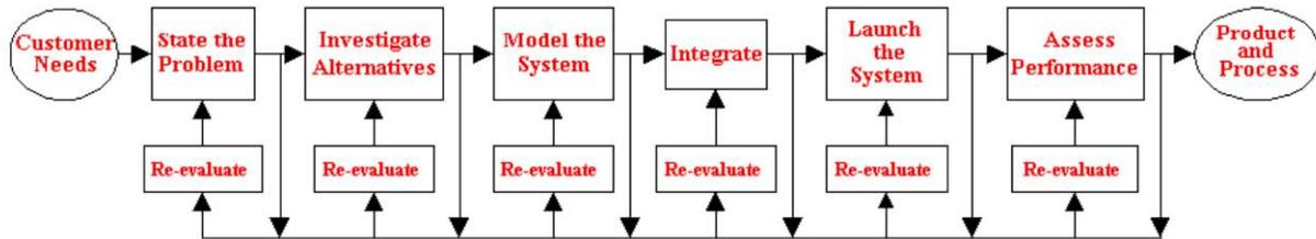
Figure 2. The SIMILAR Systems Engineering Process <sup>4</sup>
