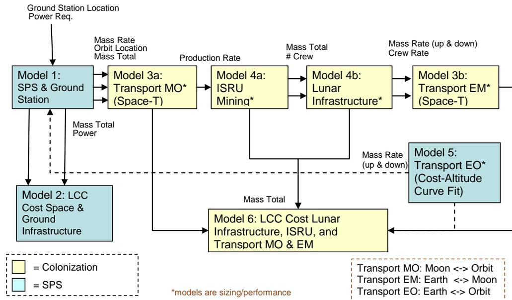
**Figure 5. The Space Solar Power model interfaces with the Lunar Colonization model to yield Solar Power Satellite masses and costs.**
