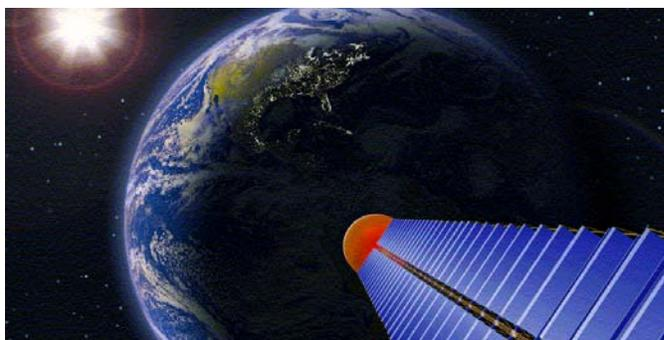
**Figure 1. A Boeing concept for a Sun Tower solar power satellite would beam power from space to Earth via low-density microwaves.**
